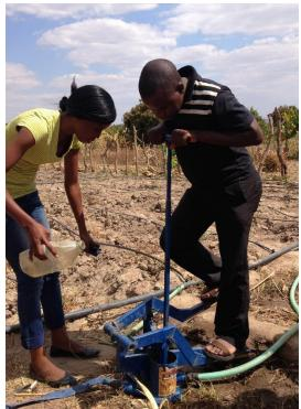
The treadle pump reduces the difficulty of irrigation. © M Messner 2015
